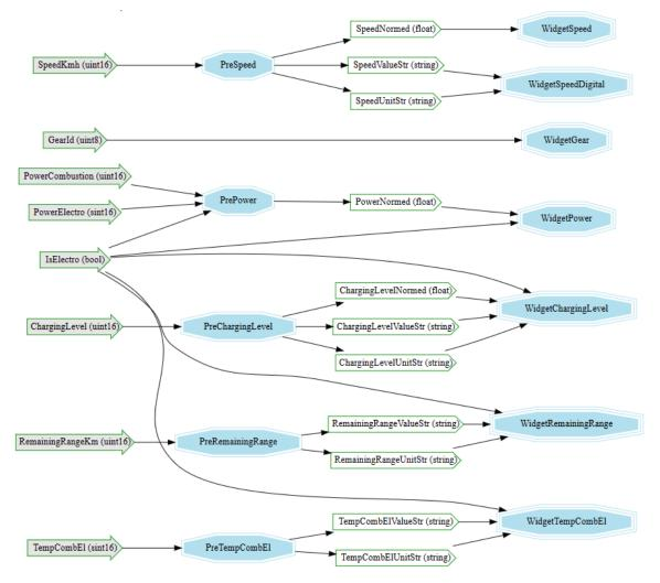
Figure 2: A part of the signal flow visualization
