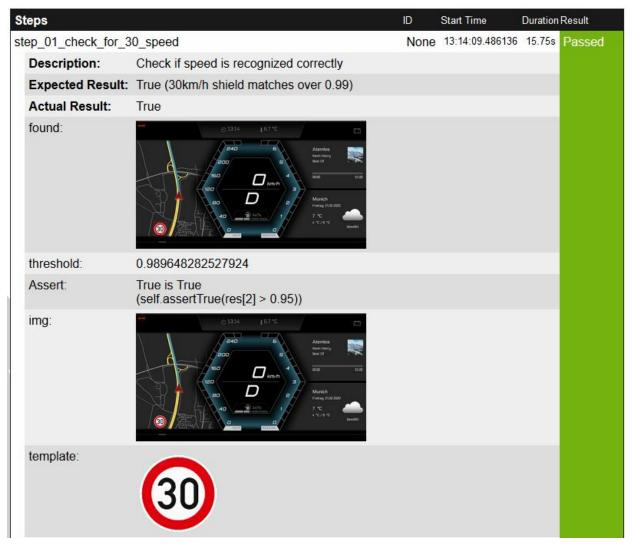
Figure 7: Test report for verification of 30 km/h speed sign
