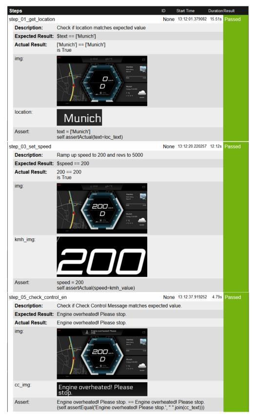
Figure 8: OCR is reading out the location, speed and control message
